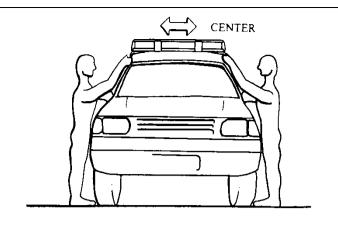
15. At this stage it is best to step back and view whether the rack is centred. As the width adjustment is not fully tightened the rack should be moved until it is centred over the vehicle. Refer to diagram shown
