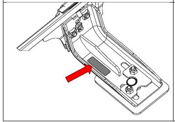
9. Place the compliance label on the rear driver's side leg in the location shown. Rub firmly to ensure adhesion.
