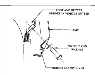
20. To complete fitment place the rubber clamp covers onto the clamps. Fasten the rack to the vehicle gutters using the rubber covered clamps and M8 x 30mm socket head bolts and washers. The bolts pass through the slots in the clamps into the captive nuts in the feet. This pulls the clamps both up and into the vehicle gutter. Excessive over tightening of these bolts may result in damage to the vehicle gutter.
